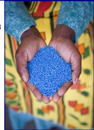
Master batch of granules containing permethrin and the polyethylene-based formulation technology.
